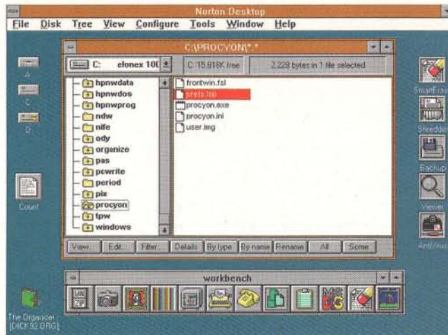
Screen 3: This Norton Desktop screen shows examples of drive icons, desktop icons for commonly used tools like SmartErase, and a toolbox view of the Quick Access window that I have named Workbench.
